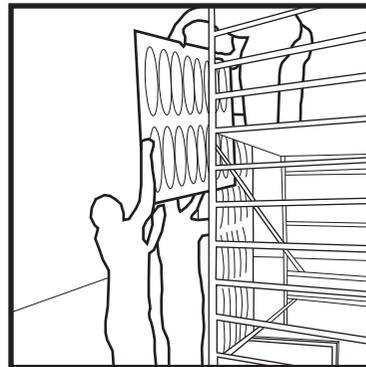
11. Remove the third module from inside the box and insert it on its position. For this operation, you will need a double-flight scaffolding.
