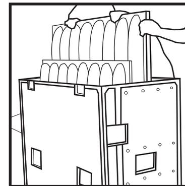
*3. Remove the first module from inside the flight-case.*
