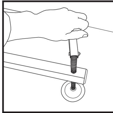
8. Check again that the three threaded feet are well adjusted and leveled.
